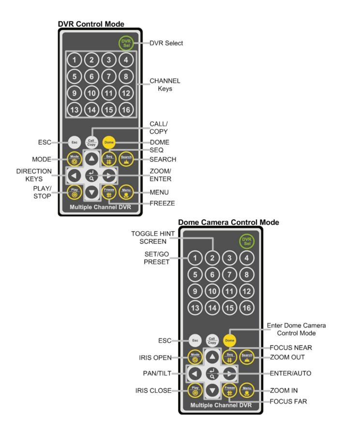
The keys of the remote control function as the keys of the front panel of the DVR. The only difference between the remote control and the front panel keys is the "DVR SEL" key. The DVR Selection key is used to switch control between each DVR.
