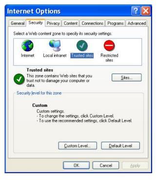
Uncheck "Require server verification (https:) for all sites in this zone". Type the IP address of the unit in field and click <Add> to add this web site to the zone.
